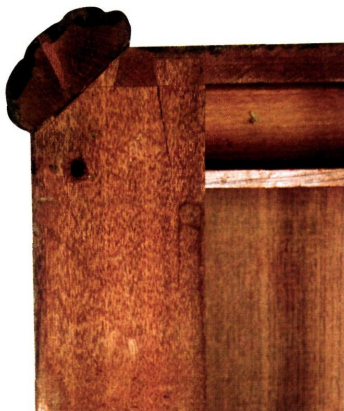
Plate 1b. A view with the top of the chest removed to show the construction of the corner columns. It is impossible to turn this shape which is asymmetric when seen from above.
