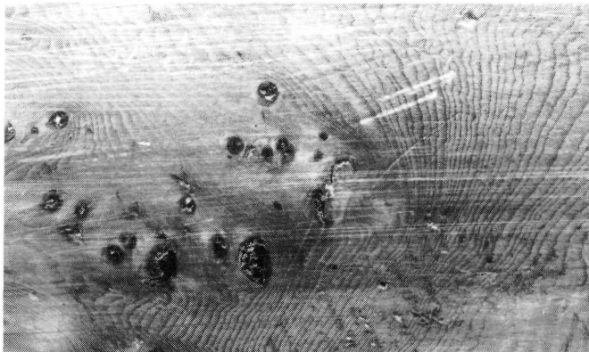
Plate 14. Huon Pine with bark inclusions in the knots and closely spaced early wood, late wood figure.
