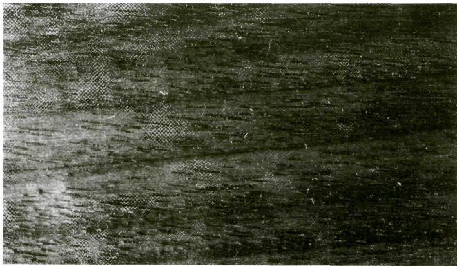
Plate 13. Blackwood; note dark bands and evenly spread pores.
