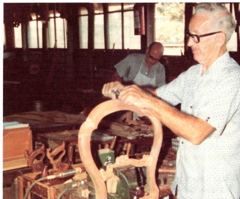
Cabinetmaker tradesman spoke-shaving the back rail of a 'Glen' dining chair
